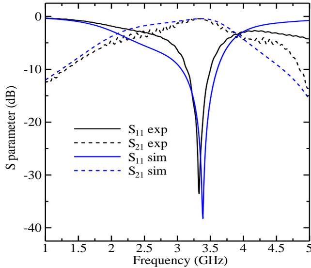
**Fig. 3.** The experimental and simulated reflection/transmission coefficients of the sensor.
