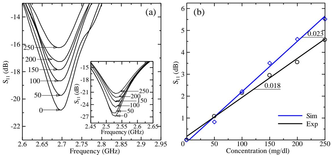
**Fig. 4.** (a) Simulated and measured (inset) results of microwave reflection coefficient  $S_{11}$  profile for DI water and for glucose aqueous solution with different concentrations 50-250 mg/dl for 500  $\mu\text{l}$  volume. (b) The simulated and measured microwave response dependence on D-glucose concentration at the resonant frequency of about 2.67 GHz and 2.53 GHz, respectively.
