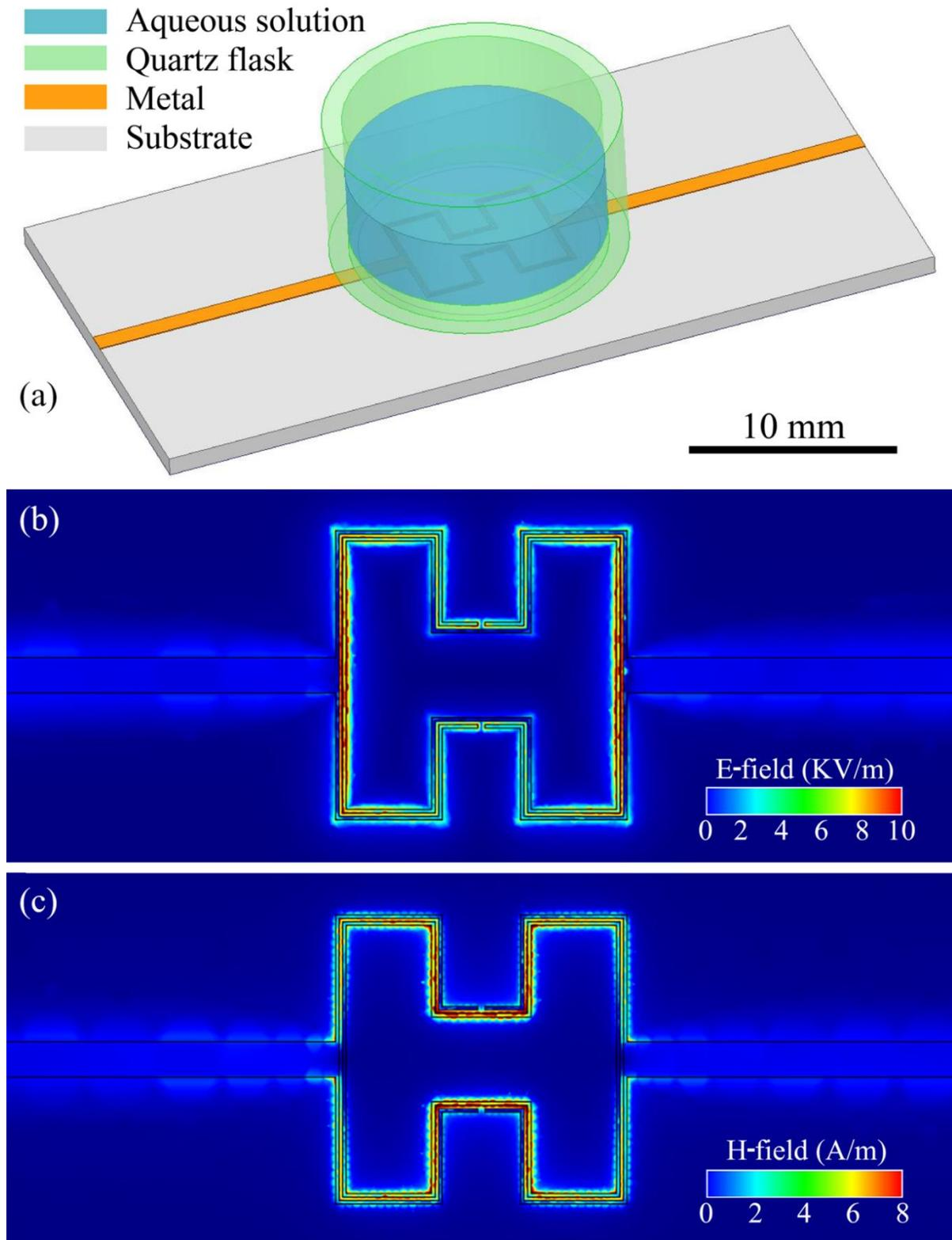
**Fig. 2.** (a) The geometry of the sensor simulation model in COMSOL. Simulated (b) electric and (c) magnetic near-field distribution at 3.3 GHz.
