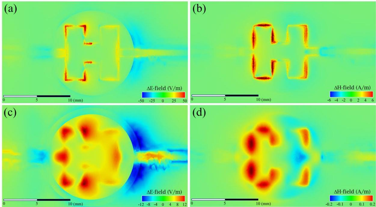
**Fig. 5.** The simulated subtraction image of 250 mg/dB and 0 mg/dl (DI water) MUTs for (a), (c) electric field and the (b), (d) magnetic field at (a), (b) sensor/MUT interface (i.e. on boundary of sensor/glucose solution) and (c), (d) at 1 mm distance from sensor/MUT interface (i.e. inside of the glucose solution), respectively at an operating frequency 2.67 GHz.
