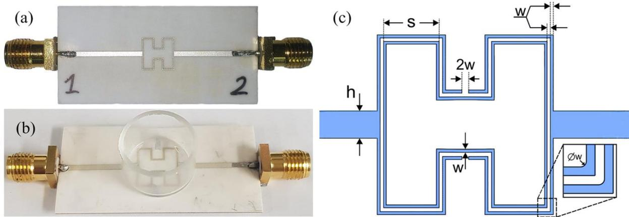
**Fig. 1.** The modified 1<sup>st</sup> order Hilbert-shaped fractal sensor (a) without and (b) with quartz vial. (c) The structural geometry of sensor pattern.
