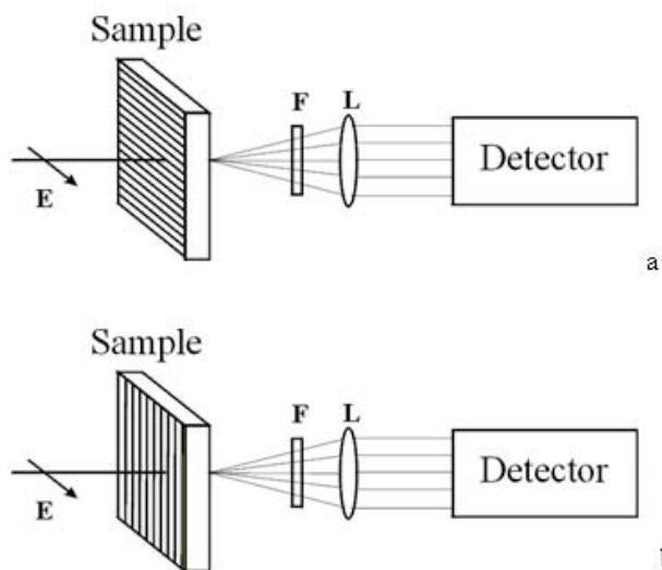
**Fig. 2.** Two cases of irradiation of samples: (a) polarization of laser beam was parallel to collagen fibers; (b) polarization of laser beam was perpendicular to collagen fibers.
