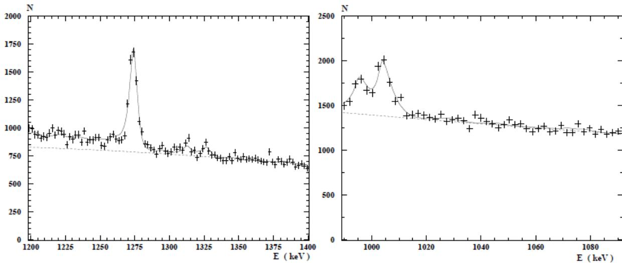
Figure 3 (left). The detector response function in the registered energy range of 1200÷1400 keV in the measurements with the source. The solid curve is the fit result (see the text). The dashed line is the fitted background.
