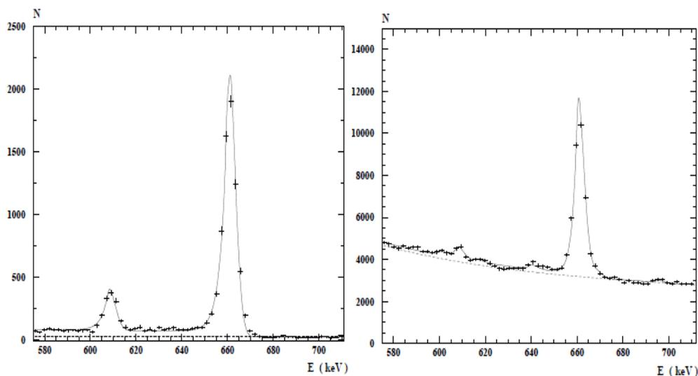
Figure 1 (left). The detector response function in the registered energy range of 575÷710 keV in the measurements with the source container. The solid curve is the fit result (see the text). The dashed line is the fitted background.
