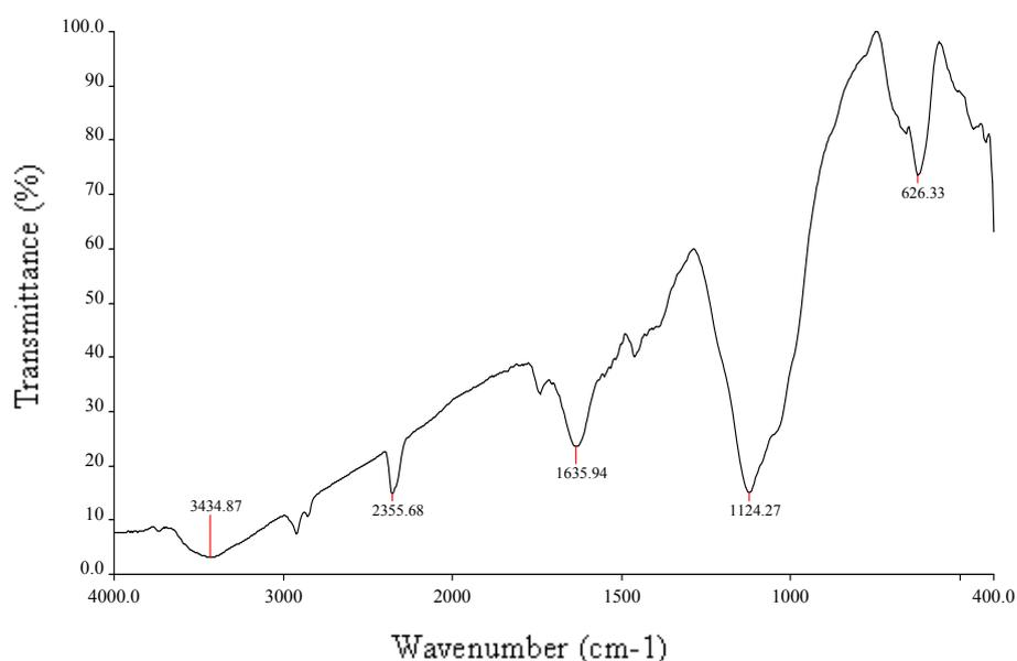
Fig. 7. FTIR spectrum of CdSe/Polythiophene nanocomposite.
