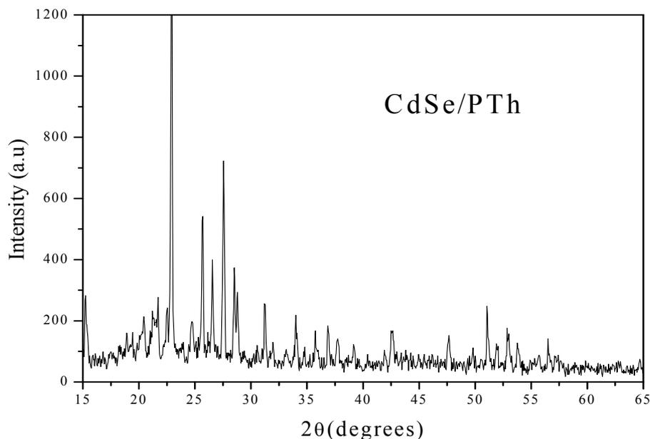
Fig. 3. XRD pattern of CdSe / Polythiophene nanocomposite.
