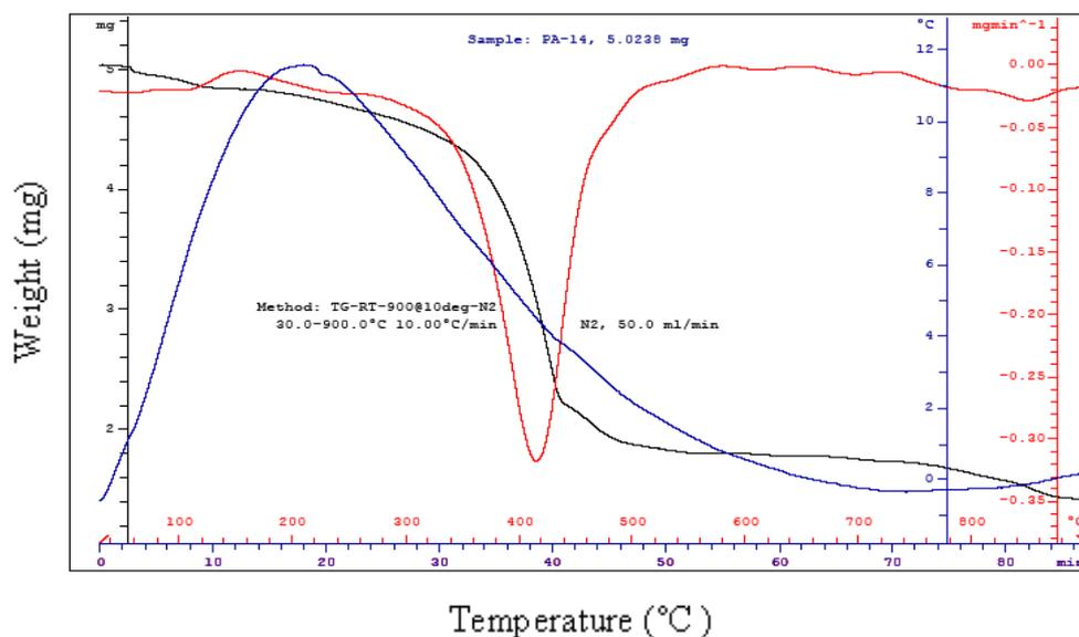
Fig. 2. TGA/DTA of CdSe/Polythiophene nanocomposite.
