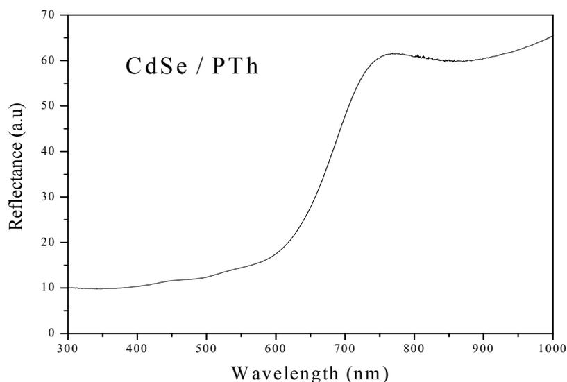
Fig. 4. UV-VIS spectrum of CdSe / Polythiophene nanocomposite.
